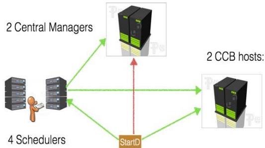
Figure 4. The final recommended HTCondor topology for deployments in order to run more than 100k parallel running jobs.
