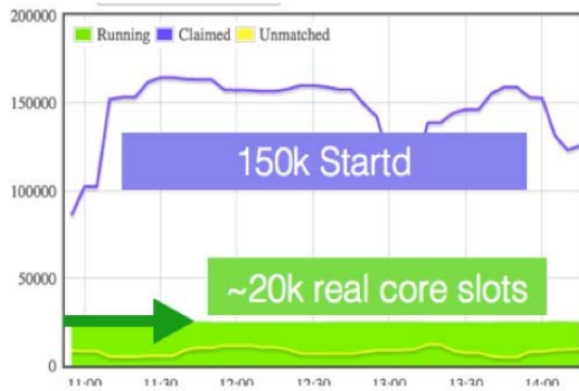
Figure 2. Uber GlideIn providing 150k sleep slots while only using 20k real cores.
